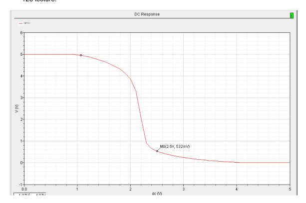
Because our NMOS and PMOS have different resistance values when they are "ON" when x=2.5 volts, y is not equal to 2.5. We must change the size of our devices to make the "ON" resistance of the PMOS and NMOS equal for our inverter. We will do this by using a "parametric" analysis to help us size our devices.
