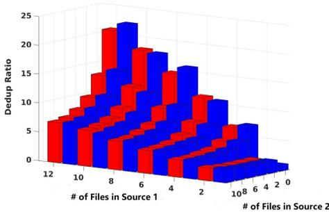
Fig. 2: The difference on real dedup ratio and the estimated one is less than 4%.
