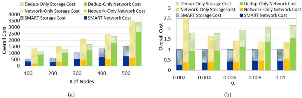
Fig. 7: Simulations on larger network size and varying values of the trade-off factor  $\alpha$  confirm that EF-dedup outperforms other algorithms in the aggregate cost that captures the network storage trade-off.
