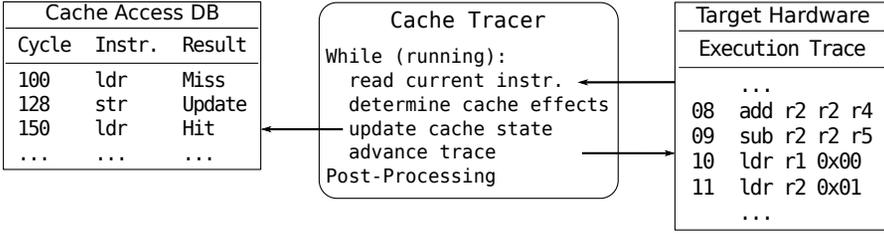
Fig. 2. The high-level design of OCD Cache Tracer has three primary components: a database to store cache accesses, the Cache Tracer program which coordinates the data collection, and the execution trace of the program on the target hardware. The primary loop of Cache Tracer is to read the current instruction of the execution, determine how that line interacts with the cache, store the results in the cache access database, and advance the execution to the next line.
