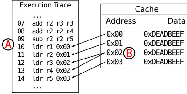
Fig. 1. This simplified program and cache diagram illustrates potential bias in injecting faults via JTAG. A: injection on the *next* load after the selected injection time will result in a disproportionate number of faults injected on line 10 compared to line 11. B: Lines 12 and 13 both read from the same address, an effect that is ignored without considering the cache state.
