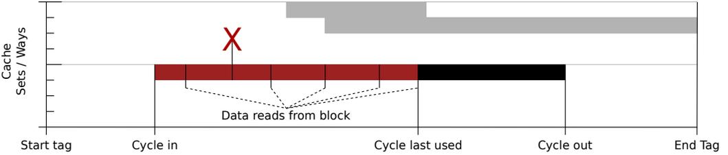
Fig. 3. The cache profile's view of critical data in the cache. The *cycle in* is recorded when data enters the cache (either via a store or load miss), and all subsequent load instructions are recorded. The last time the data is read is marked as *cycle last used*; the data is no longer critical after this point. The label *cycle out* marks when the data is evicted or overwritten by a store.
