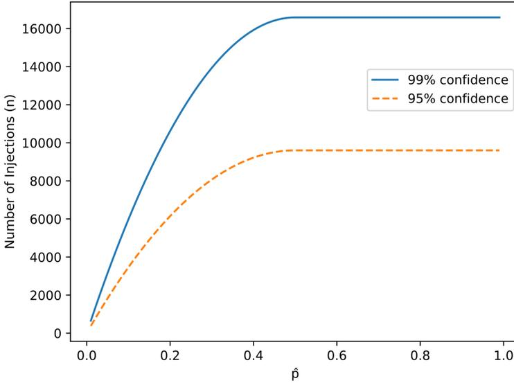
Fig. 6. The number of fault injections required (as calculated by equation 1) as  $\hat{p}$  changes. Without prior knowledge of the benchmark,  $\hat{p}$  is set to 0.5. This chart shows that the number of fault injections may be reduced when  $\hat{p}$  is set based on the critical data measurement from the cache profile.
