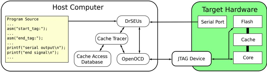
Fig. 4. An overview of the primary components needed for running OCD Cache Tracer. The host computer runs DrSEUs which uses OpenOCD/JTAG to load the test program and controls execution. DrSEUs records and monitors the test program output through a serial port. OCD Cache Tracer is integrated with DrSEUs and creates a database of cache accesses by stepping the test program's execution and monitoring cache accesses through OpenOCD/JTAG.
