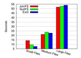
**Figure 4.** Overheads of transferring a directory hierarchy into JOINFS.
