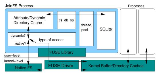
**Figure 2.** The high-level JOINFS design. The kernel buffers file data, and JOINFS passes file requests on to the native file system. Dynamic directories are handled by the logic and SQLite backend.
