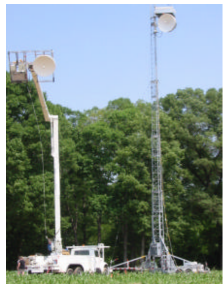
A multi-frequency, active radar system developed by GW/NASA (left) and an L-band, single-frequency radiometer (right) collect data on corn.
