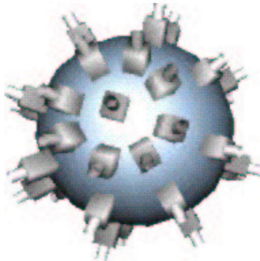
Figure 5. A compound-like eye composed of conventional video cameras.
