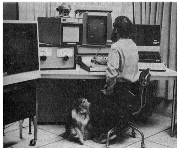
Fig. 7 The KINSYN III hardware. The human user was utilized as an integral part of the synthesis procedure. The user observed the current state of the design on the CRT screen and input directions for continuing the synthesis by way of a data tablet. (From Ref. [9]; used by permission of ASME.)
