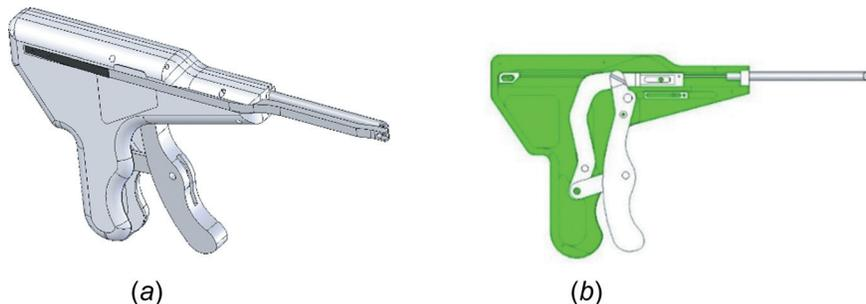
**Fig. 15 Pistol-shaped fastener deployment hand piece**
