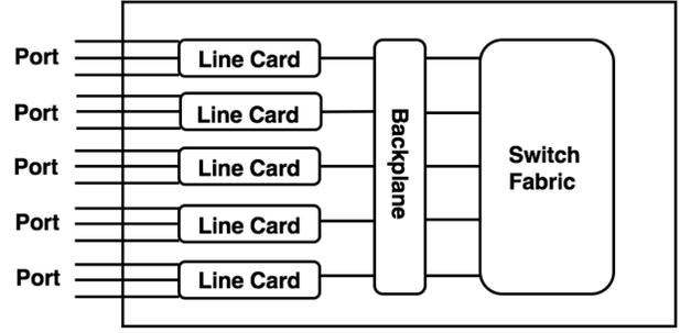
Figure 3: Schematic of switch, line card, and its ports.
