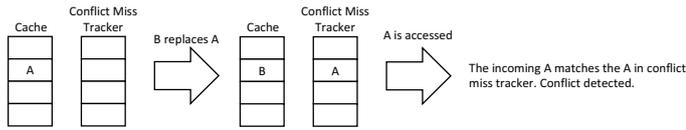
Fig. 5: The changes in cache and conflict miss tracker when a replaced memory line A is accessed again.
