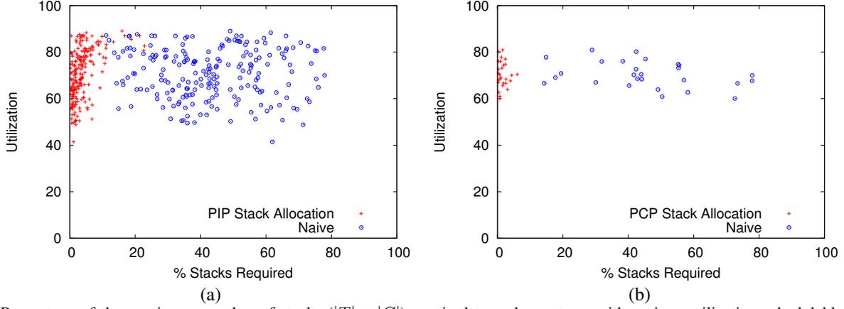
Fig. 5. Percentage of the maximum number of stacks ( $|T| \times |C|$ ) required to make systems with a given utilization schedulable that were not schedulable with  $\forall c^x, s^x = 1$ , but are with  $s^x = |T|$ . (a) Plots for the 207 (of 1K) systems that did not pass for PIP, while (b) plots the 27 (of 1K) systems for PCP. A vertical split in either graph yields the number of systems (on the left of the split) that will be schedulable given a specific percent of stacks.
