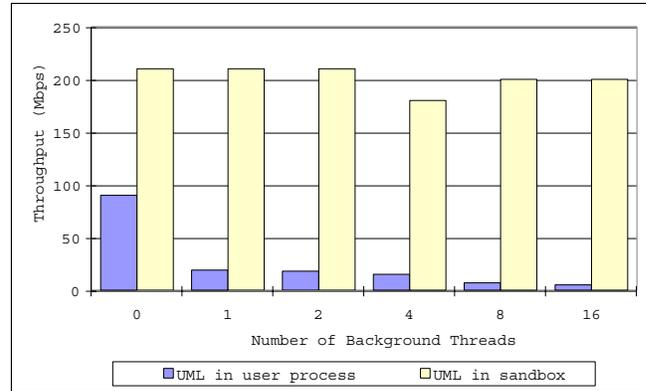
**Figure 3. Throughput comparison of UML in a sandbox versus user-process.**
