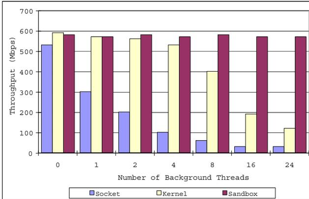
**Figure 4. Throughput comparison of an optimized sandbox stack versus both user-level sockets and kernel implementations.**
