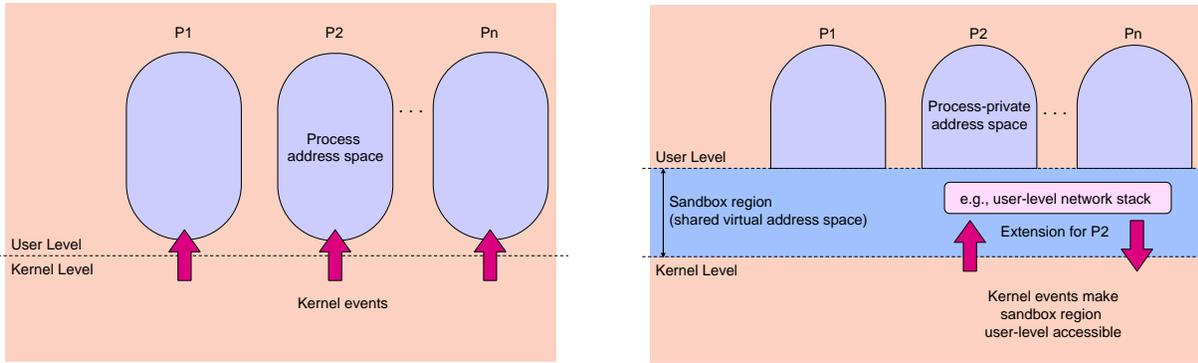
**Figure 1. (a) Traditional view of logical protection domains, each mapped to a separate address space. (b) With user-level sandboxing each process address space has a shared virtual memory region into which extensions are mapped. For example, an extension might support a network stack that is activated by kernel events when packets arrive on a network interface.**
