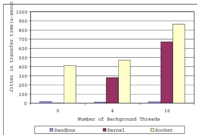
**Figure 5. Maximum jitter in transfer time.**
