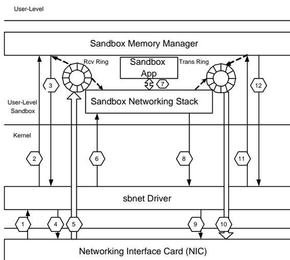
Figure 2. User-level networking in a sandbox.
