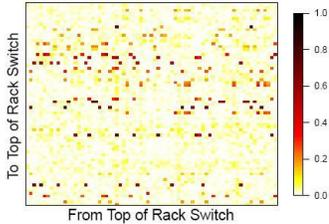
Fig. 1. Matrix of application demands between top of rack switches [6]
