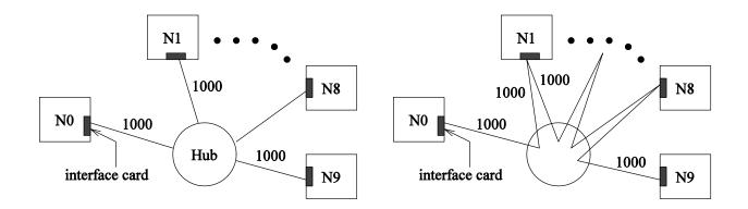
(a) The figure on the left shows a network with a hub. Each computer is connected to the hub with a cable of length 1000 m. Calculate the minimum frame size that can be supported so that CSMA/CD protocol will function correctly.
