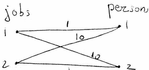
$$c_{11} = 1, c_{12} = 10, c_{21} = 10, c_{22} = 100$$
