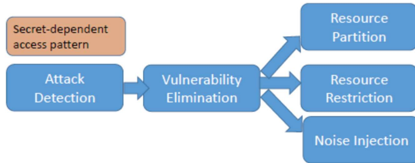
Figure 2. Attack and Vulnerability Elimination Strategies for Side and Covert Channels [Source: Adapted from Yinqian Zhang’s talk at the workshop].
