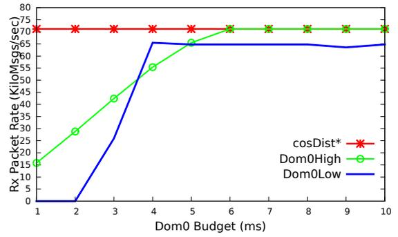
Fig. 10: Throughput measurements for IOVM running a UDP server and with smaller DLVM execution (C=0.5ms P=10ms), using a simple UDP client tool on the host.
