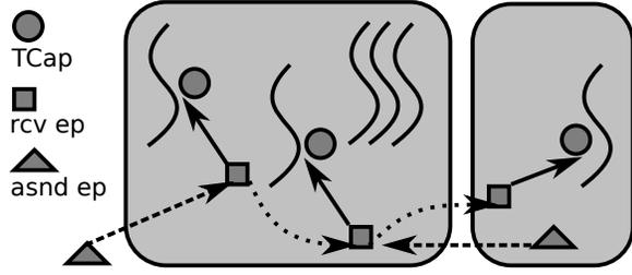
Fig. 5: TCaps data-structures, and their relationships. Solid arrows indicate the thread and TCap associated with a receive end-point. Dashed arrows show the connection between an asnd and rcv end-points. Dotted arrows indicate the scheduler thread/TCap.
