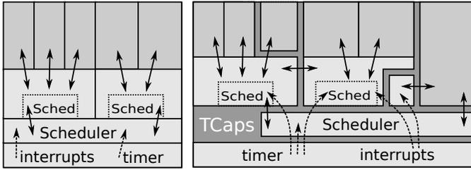
Fig. 1: Left: a traditional system with virtual machines. Applications are in darker grey at the top. Arrows designate control flow, and dotted arrows designate hardware interaction. Right: a system where the TCaps mediate and control interactions between subsystems. Darkest grey paths designate processing time flow through TCaps.
