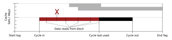
Fig. 3. The cache profile's view of critical data in the cache. The *cycle in* is recorded when data enters the cache (either via a store or load miss), and all subsequent load instructions are recorded. The last time the data is read is marked as *cycle last used*; the data is no longer critical after this point. The label *cycle out* marks when the data is evicted or overwritten by a store.
