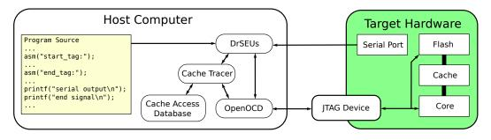
Fig. 4. An overview of the primary components needed for running OCD Cache Tracer. The host computer runs DrSEUs which uses OpenOCD/JTAG to load the test program and controls execution. DrSEUs records and monitors the test program output through a serial port. OCD Cache Tracer is integrated with DrSEUs and creates a database of cache accesses by stepping the test program's execution and monitoring cache accesses through OpenOCD/JTAG.
