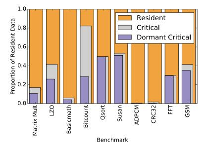
Fig. 5. Critical and dormant critical data shown as a proportion of total resident data (height is scaled proportionally; width is scaled to show subset relationship)
