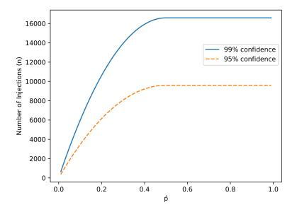
Fig. 6. The number of fault injections required (as calculated by equation 1) as  $\hat{p}$  changes. Without prior knowledge of the benchmark,  $\hat{p}$  is set to 0.5. This chart shows that the number of fault injections may be reduced when  $\hat{p}$  is set based on the critical data measurement from the cache profile.
