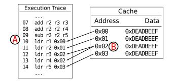
Fig. 1. This simplified program and cache diagram illustrates potential bias in injecting faults via JTAG. A: injection on the *next* load after the selected injection time will result in a disproportionate number of faults injected on line 10 compared to line 11. B: Lines 12 and 13 both read from the same address, an effect that is ignored without considering the cache state.
