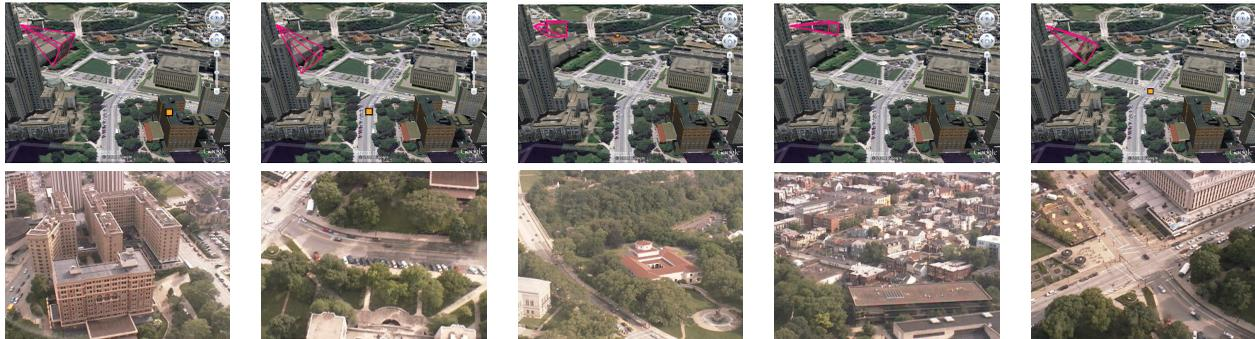
Fig. 12. Examples of a geographically-aware PTZ interface. (Top row) A user drags the orange query point around the virtual 3D environment. We find the optimal pan and tilt values that orients the camera toward the query point and (bottom row) remotely control the physical camera to match those orientation parameters. In each example, the camera is controlled entirely by the manipulation of the orange point in Google Earth.
