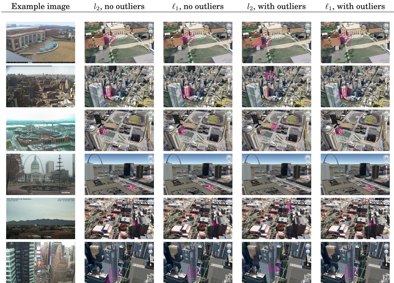
Fig. 4. Each row shows an example image of the camera, and the results from both the least squares approach ( $l_2$ ) and the robust calibration method ( $l_1$ ) in the absence and presence of outliers. The proposed algorithm consistently returns more robust calibrations than traditional methods. In the fourth row, the least squares approach placed the camera kilometers away from the ground truth location and is not shown.
