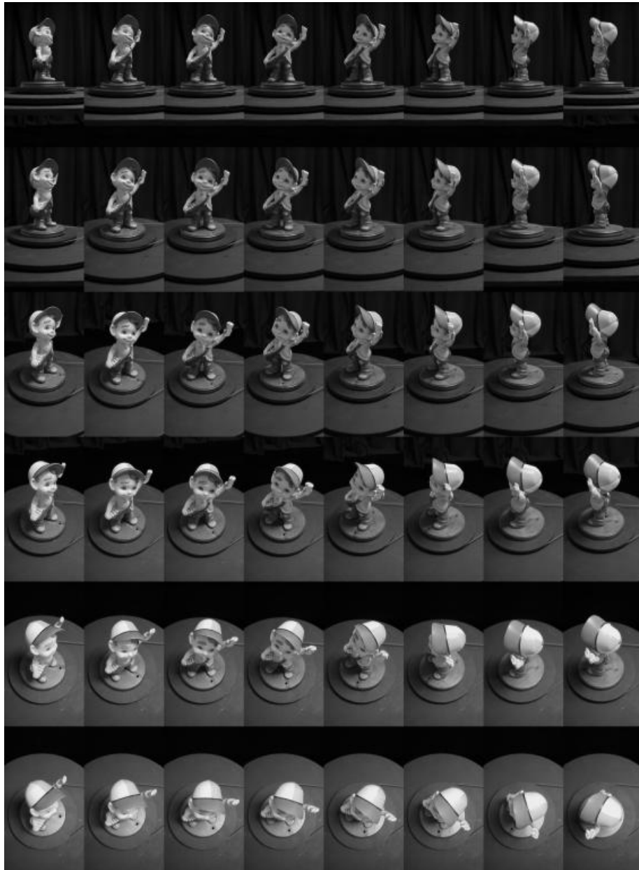
Figure 5: Images from an even sampling of the final embedded space shown in Figure 4, (bottom right). The mean embedding error over all 1800 images is only 6.98^\circ for the rotation, and 2.97^\circ for the camera elevation.
