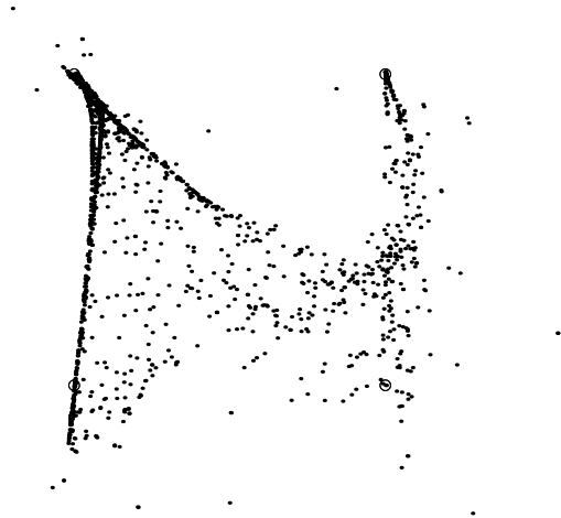
Figure 3: Locally Linear Embedding: Each image was expressed as a linear combination of nearby images. The points were embedded with the additional constraint that the four corner images lie at fixed positions at the corner of a square.
