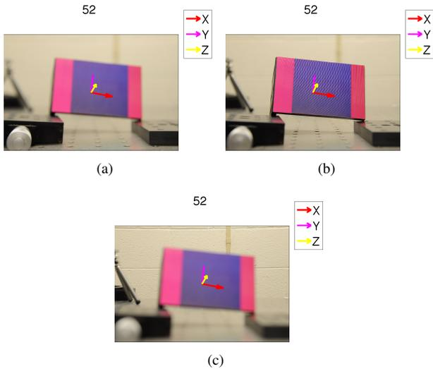
Figure 11. Our rotation estimation object works even for out of focus images. For each image, we show the rotation estimate as a set of axis. We show the results for images a) focused in front, b) focused on, and c) focused behind the calibration object.
