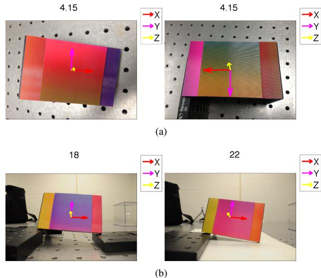
Figure 10. We estimate camera rotation from various poses and focal lengths. In the first row, we show calibrated images taken by an iPhone for different orientations of the calibration object. In the second row, we show calibrated images of images taken by a Nikon D90 DLSR with varying focal lengths. For each image, we show the focal length in the title and the rotation of the local axis of the calibration object superimposed on the image.
