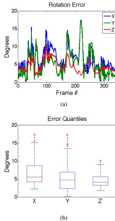
Figure 8. For a test video with varying camera orientations, we test the rotation accuracy of our prototype. We show the rotation error for each frame of the video in a) and summary statistics in b).
