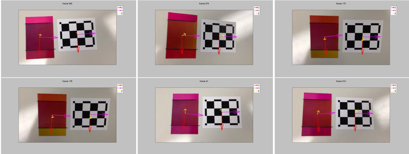
Figure 9. We show random frames from a video used to assess the rotation accuracy of our prototype structured light field. As an Augmented Reality Application, we overlay representations of the local axes. We do this for both our prototype and the ground truthing checkerboard to visually assess rotation estimation accuracy.
