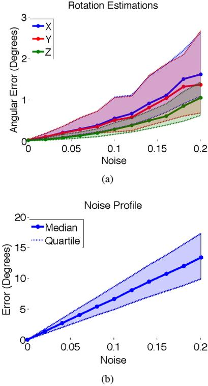
Figure 5. As more noise is introduced to  $\vec{n}_{hue}$ , the a) rotation error for all axes increases and is less consistent. b) shows the quartiles of angular error introduced to  $\vec{n}_{hue}$  for a given standard deviation of noise.
