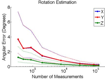
Figure 6. Using more measurements, and thus geometric constraints, in the optimization results in a lower and more consistent rotation error.
