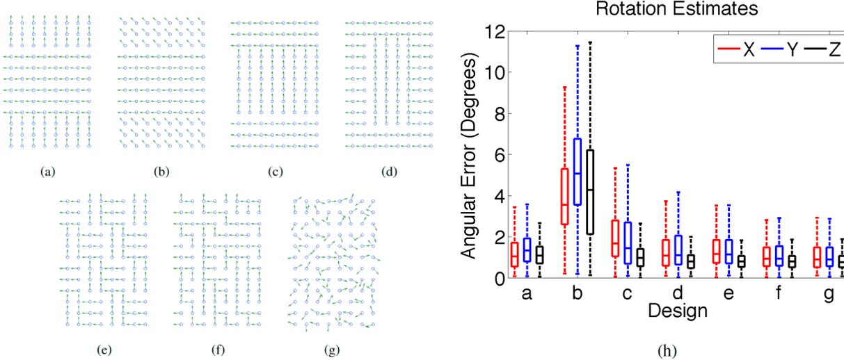
Figure 7. Various designs (a-g) change the orientation and relative positions of lenticular arrays to make a calibration object. Estimations achieved for design g) have the lowest h) rotation error, however it is an unrealistic design. c) is a more reasonable design.
