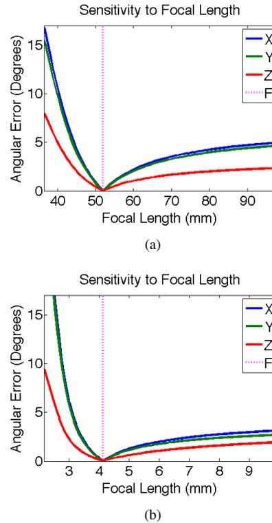
Figure 12. We explore the optimization of the rotation separately for two images (from Figures 10(a) (the right) and 11(b)). For both images, we vary the focal length of the camera calibration matrix used in our constraints and observe the effects on rotation estimation. Even for relatively large focal length errors, the rotation estimation has less than 5 degrees of error.
