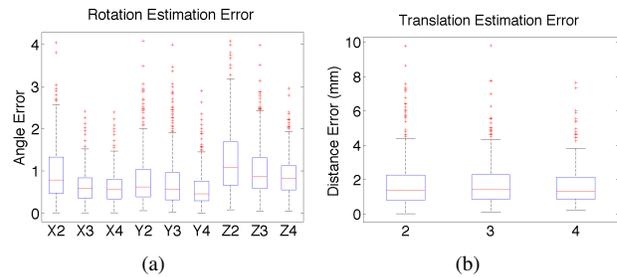
Figure 6. Although two lenticular markers are sufficient to constrain the pose estimation problem, using more lenticular markers improves rotation performance. Here we show the performance effects of increasing the number of lenticular markers in a) rotation estimation and b) translation estimation.
