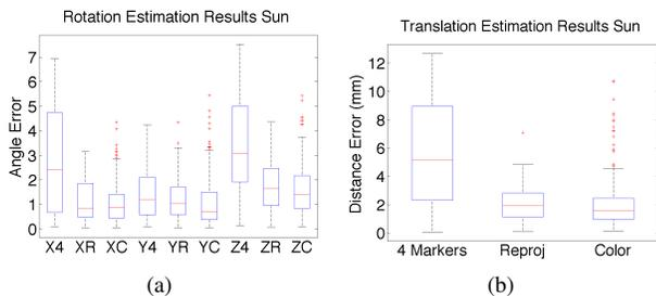
Figure 7. Optimizing for reprojection error and color calibration variables mitigates the negative effects of a lighting environment very different from calibration, such as full sun shown here. The a) rotation error reduces for each axis and b) the translation error reduces with the reprojection color calibration routine.
