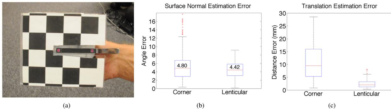
Figure 4. We compared lenticular fiducial markers with the state of the art “corner” method on a video (of which an example frame is shown in a). For the length of the video, the pose estimation using lenticular markers produces a better normal direction estimation (b) and position estimation (c) median with a much more compact distribution. Each box in b) contains the median value in text.
