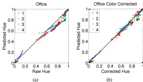
Figure 9. For a video in an office next to a window, we show color calibration results. On the left, we see the observed hue differing from the hue predicted by the HRF for the known orientations. On the right, we see that color corrected hues match the predicted hue and thus provides robustness for pose estimation in varying lighting environments.
