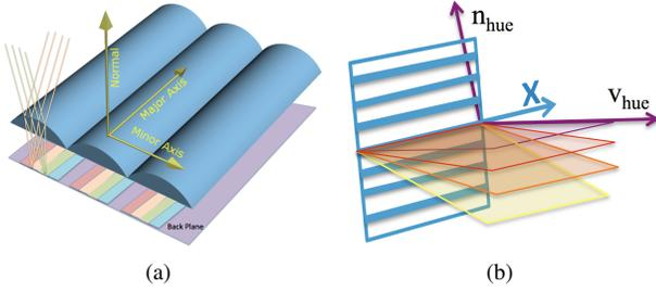
Figure 2. (a) The top surface of a lenticular array is comprised of parallel cylindrical parts that focus parallel rays onto particular rows of a backplane. (b) Relative to the major axis  $x$ , any view  $v_{hue}$  of the lenticular array with a particular hue, lie on a plane denoted by its surface normal  $n_{hue}$ .
