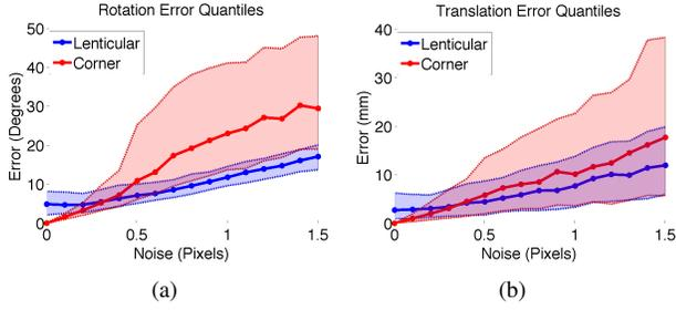
Figure 10. By using lenticular fiducial markers instead of the typical 4 corner markers, we achieve ameliorated pose estimations for rotation (a) and translation (b). In both figures, we increase the amount of error simulated along the x-axis, and show the median value for each simulation surrounded by the 1st and 3rd quantile.
