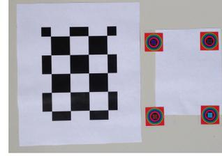
Figure 5. With a setup that mounts 4 lenticular markers on the same plane as a checkerboard, we can ground truth experiments that explore pose estimation results for more than 2 markers and color calibration routines.
