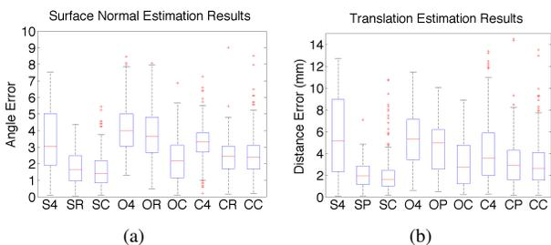
Figure 8. Despite these varying lighting conditions, reprojection optimization with color calibration produces results with very high accuracy and precision in a) surface normal estimation and b) translation estimation. Sunny, Office, and Cloudy datasets are denoted by S, O, and C respectively and 4, P, and C correspond to the three optimization routines discussed in Section 7.2.
