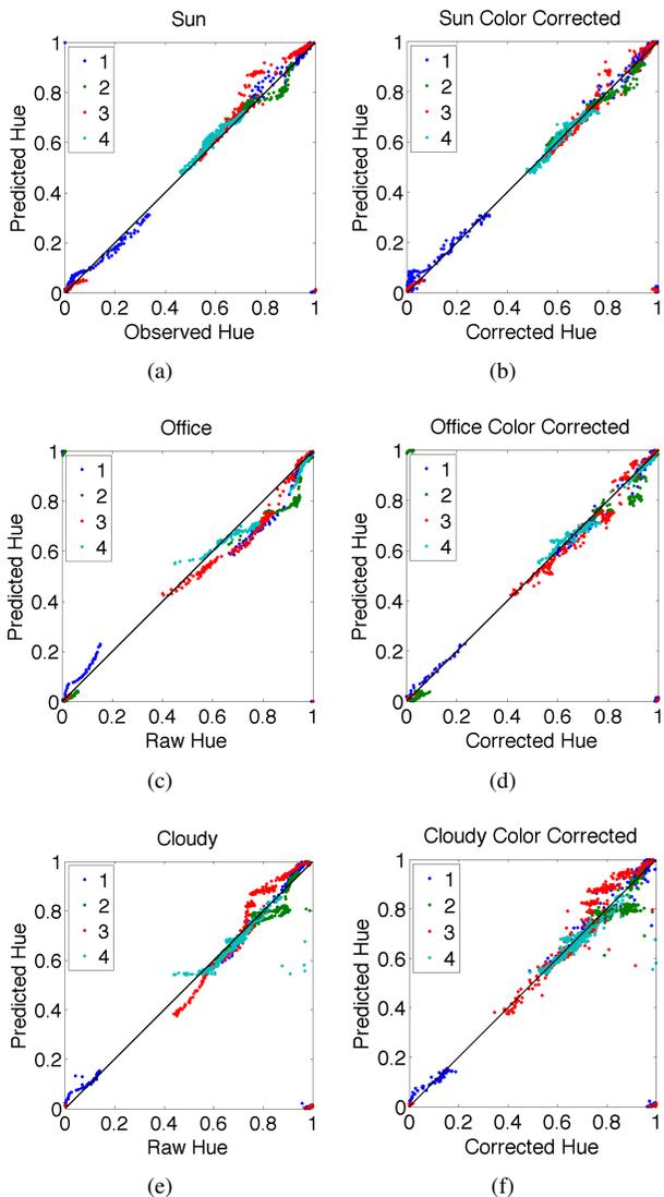
Figure 11. For three different lighting environments, we show color calibration results. In the left column, we see the observed hue differing from the hue predicted by the HRF for the known orientations. In the right column, we see that color corrected hues match the predicted hue and thus provides robustness for pose estimation in varying lighting environments.
