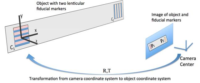
Figure 3. A pinhole camera (right) sees an image of an example flat object (left), which has two lenticular patches. The pose estimation problem asks to solve for the  $R, T$  describing the rotation and translation mapping the coordinate system of the camera to the coordinate system of the object.
