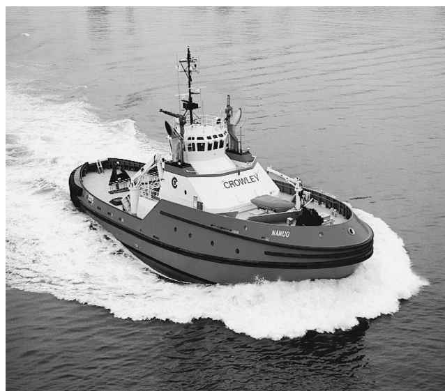
Figure 7: The 153-foot, 10,000 horsepower, state-of-the-art tractor-tug Nanuq has been put in service to escort tankers through Valdez Narrows.
