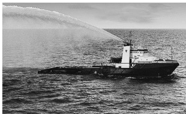
Figure 8: The enhanced capability tug Gulf Service has been stationed at Hinchinbrook Entrance to save disabled tankers even in extreme environmental conditions.
