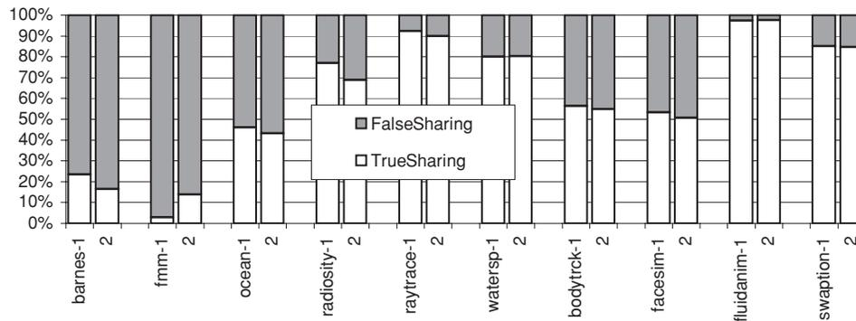
Fig. 9. Breakdown of coherence misses. For each benchmark, the two bars represent breakdown of coherence misses on caches that (1) always replace LRU block, and (2) prioritize invalid blocks over LRU block.
