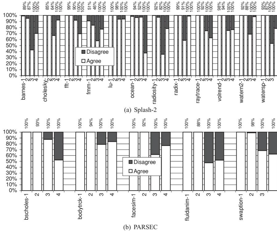
Fig. 17. Accuracy for low-cost DeFT and Dubois et al.'s schemes with classification rates (% of coherence misses that are actually classified) shown above each bar. For each benchmark, bar 1 (leftmost bar in each 4-bar group) represents (Partial (16k) AcT, Partial (1k) OD), bar 2 is (Partial (4k) AcT, Partial (256) OD), bar 3 is (Zero AcT, Zero OD), and bar 4 is Dubois et al.'s scheme.
