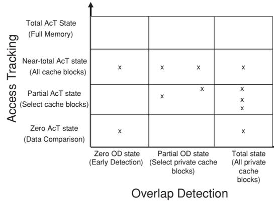
Fig. 7. Design space for coherence miss classification mechanisms. Design points marked “x” are examined in our evaluations.
