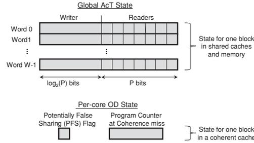
Fig. 4. State maintained and used by our I-FSD coherence miss classification algorithm.
