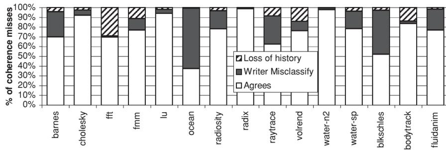
Fig. 6. Comparison between I-FSD and Dubois et al. Each bar has three portions- bottom portion shows the percentage agreement between the two schemes, and the middle and top portions show the percentage breakdown of disagreement between the two schemes.
