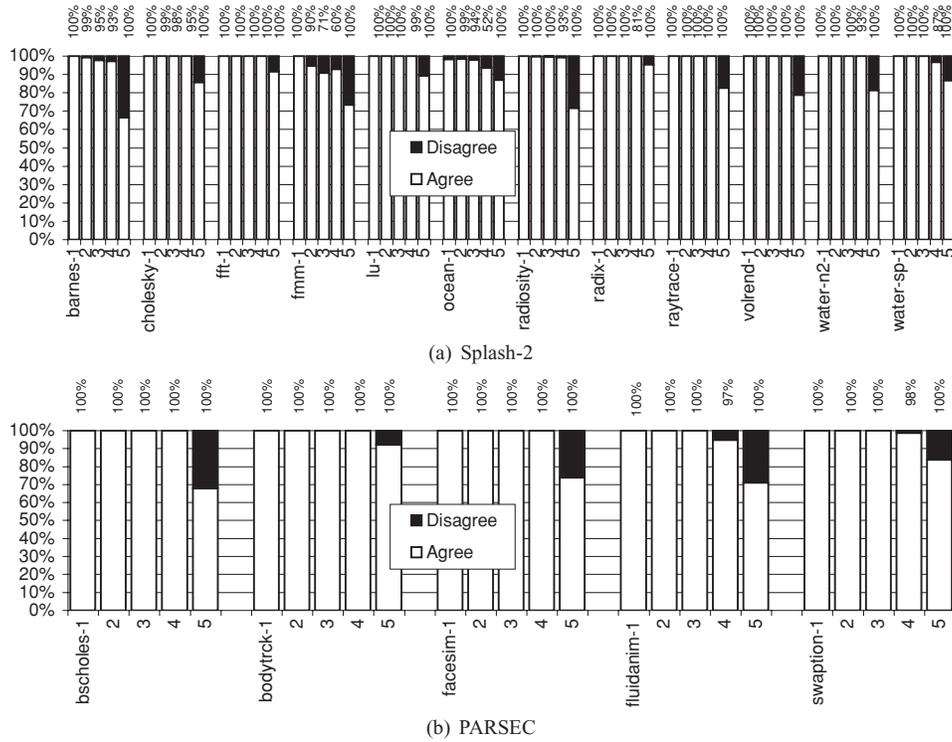
Fig. 11. Accuracy for different AcT approximations with classification rates (% of coherence misses that are actually classified) shown above each bar. For each benchmark, the five bars (from left to right labeled 1 through 5) represent Near-Total AcT state, Partial AcT state with 16k, 4k, 1k entries and Zero AcT state.
