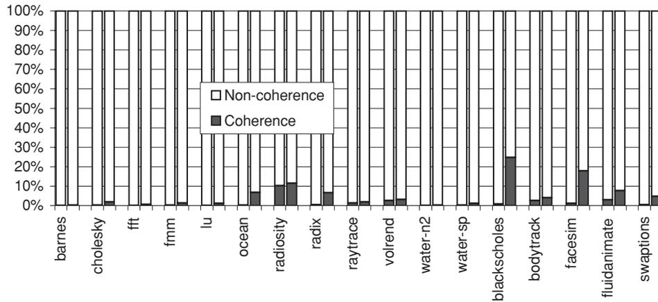
Fig. 10. Breakdown of all cache misses for 8 and 64 cores.
