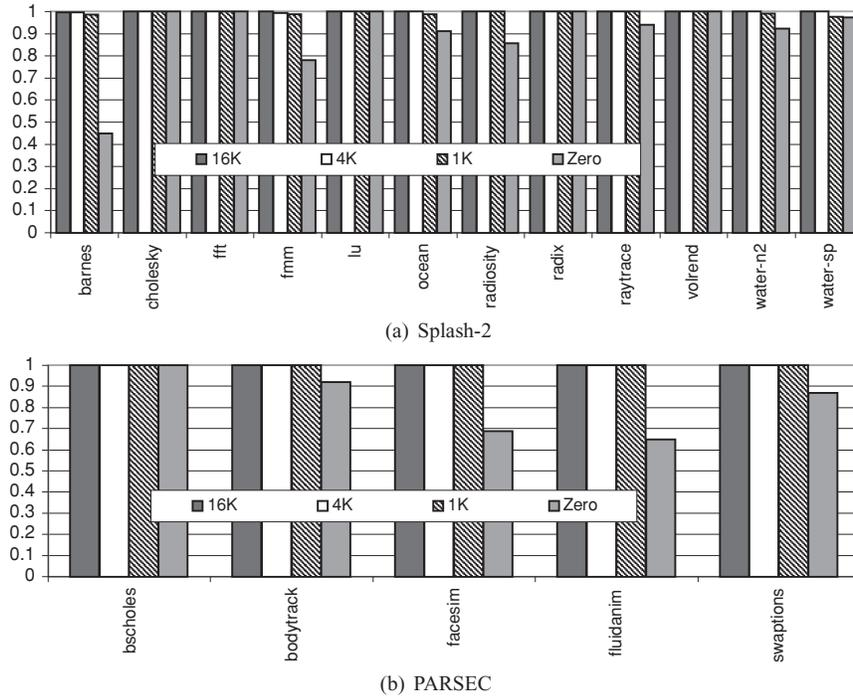
Fig. 12. Correlation coefficient between number of false sharing misses suffered by static instructions in Partial AcT, Zero AcT schemes against Near-total AcT. Samples of static instructions are chosen by Partial AcT schemes.
