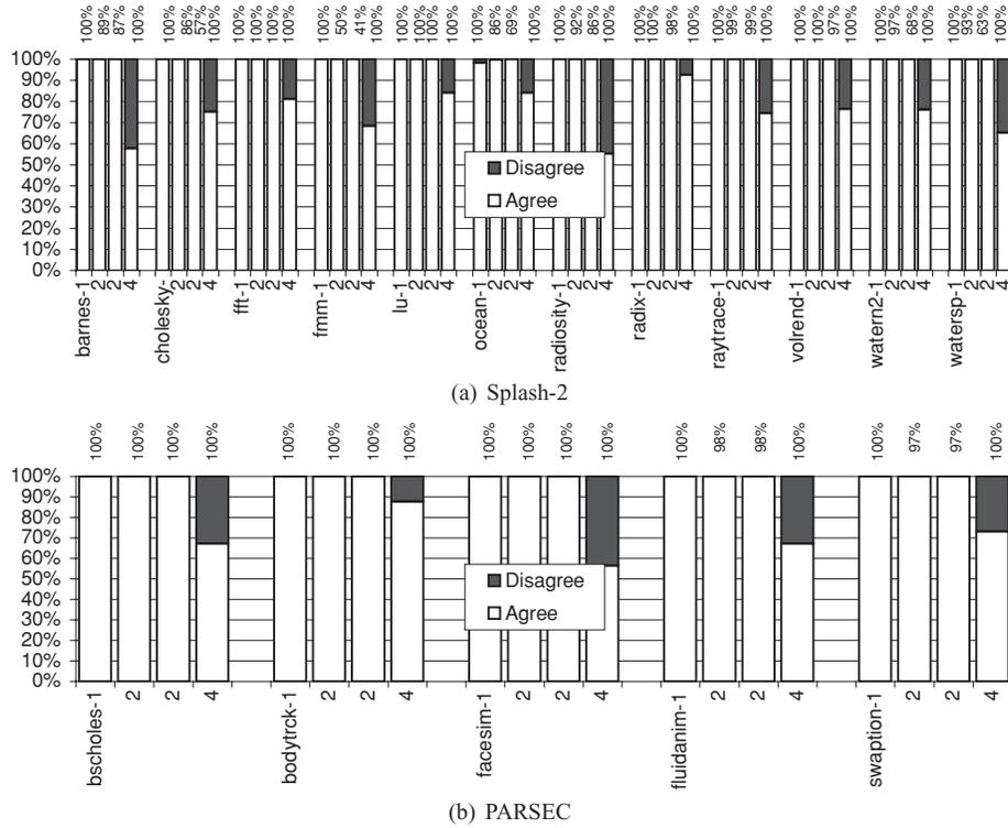
Fig. 14. Accuracy for different OD approaches with classification rates (% of coherence misses that are actually classified) shown above each bar. For each benchmark, the four bars (left to right labeled 1 through 4) represent Total OD state, Partial OD state with 1k and 256 entries, and Zero OD state.
