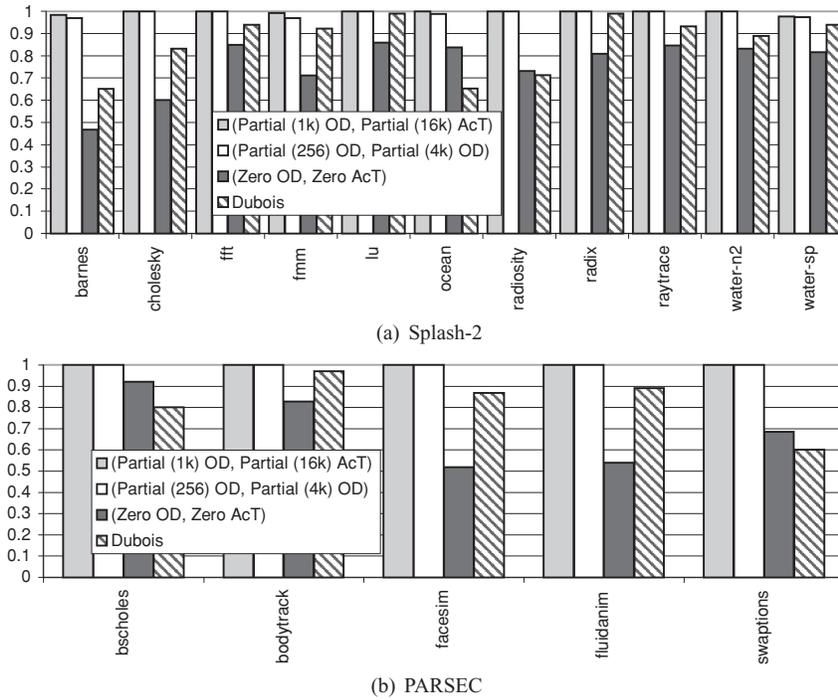
Fig. 18. Correlation coefficient between number of false sharing misses suffered by static instructions in various schemes against (Total OD, Near-Total AcT). Samples of static instructions are chosen by partial state schemes.
