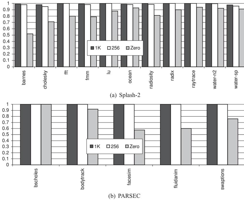
Fig. 15. Correlation coefficient between number of false sharing misses suffered by static instructions in Partial OD, Zero OD schemes against Total OD. Samples of static instructions are chosen by Partial OD schemes.
