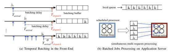
Fig. 4: An illustration of temporal job batching procedure assuming that the server is equipped with a 4-core processor. (a) shows how the jobs are batched together before they are dispatched; (b) illustrates how the batched jobs are serviced at the local server. Note that the first 4 jobs are processed simultaneously while the other jobs are queued.<sup>3</sup>
