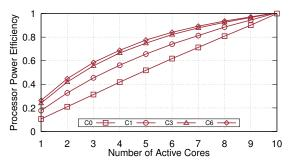
Fig. 2: Power efficiency of a 10-core Xeon processor with different level of C states configurations.
