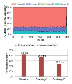
(b) Normalized energy for baseline and simple batching mechanism.
