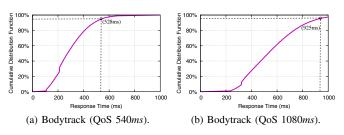
Fig. 7: Latency CDF for Bodytrack under 30% utilization using Temporal Batching.
