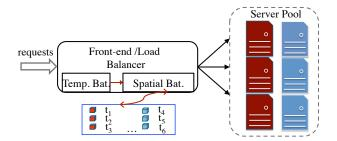
Fig. 5: Overview of overall TS-Bat scheme.  $t_i$  is the estimated processor idle time for server *i*.  $t_1$ ,  $t_2$  and  $t_3 \ge t_{cur}$ , which means these servers are currently busy processing the batched jobs;  $t_4$ ,  $t_5$  and  $t_6 \le t_{cur}$  indicating these three servers are idle.
