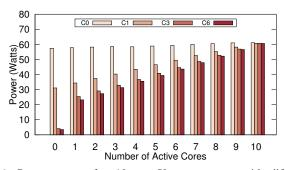
Fig. 1: Power range of a 10-core Xeon processor with different number of active cores and various C states configurations.<sup>1</sup>
