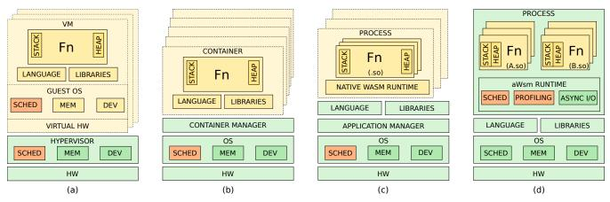
Fig. 1: (a) VM-based serverless. (b) Container-based serverless. (c) Native WASM-based serverless implementation. (d) aWsm approach for efficient serverless execution at the Edge. (*Yellow color* indicates the serverless function sandboxes, *Green color* represents shared layers and services between sandboxes in different approaches, and *Orange color* reflects control modules used for function performance management: scheduling and profiling.)
