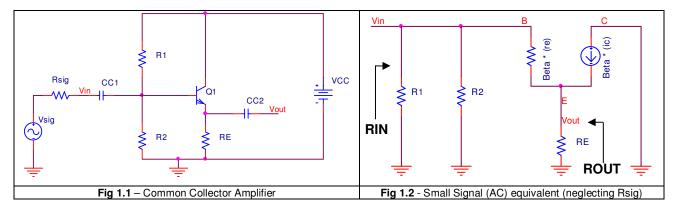
From the AC equivalent of the common-collector amplifier in figure 1.2, we can derive the input impedance, output impedance, and voltage gain:
