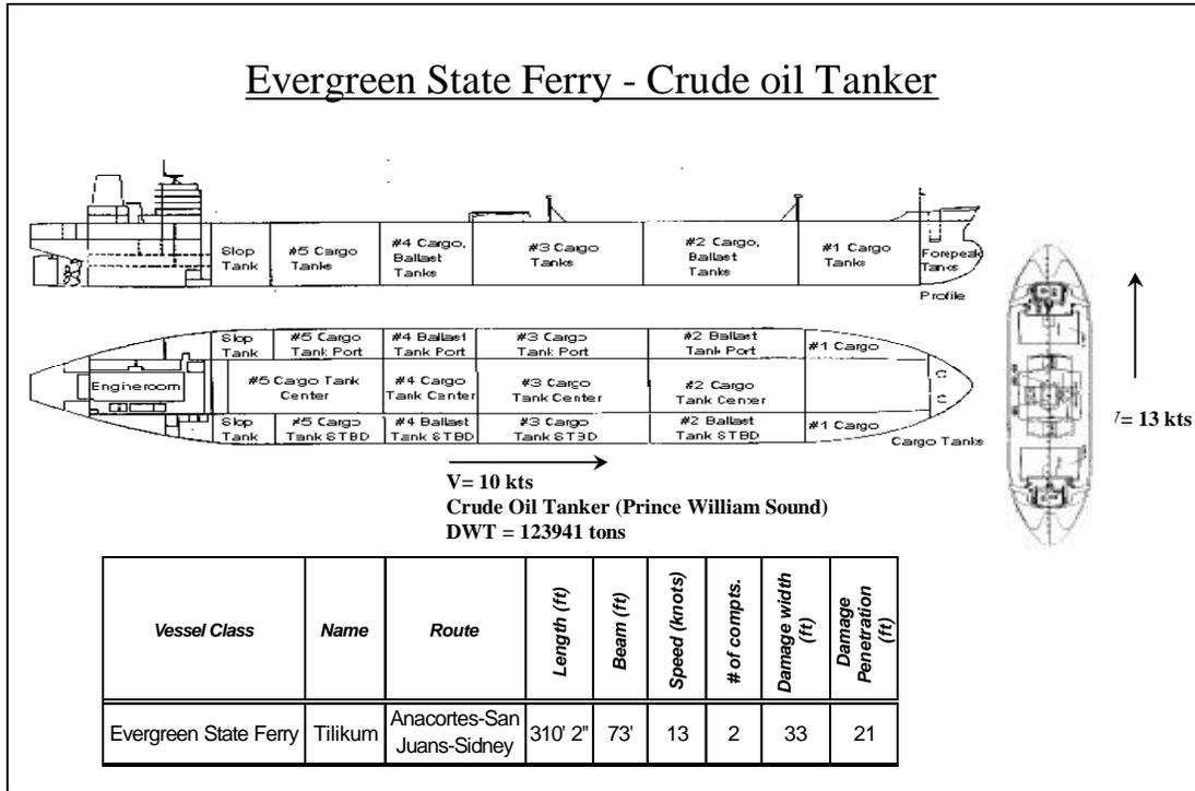
**Figure 12. A collision damage calculation based on a collision scenario with a crude oil tanker**
