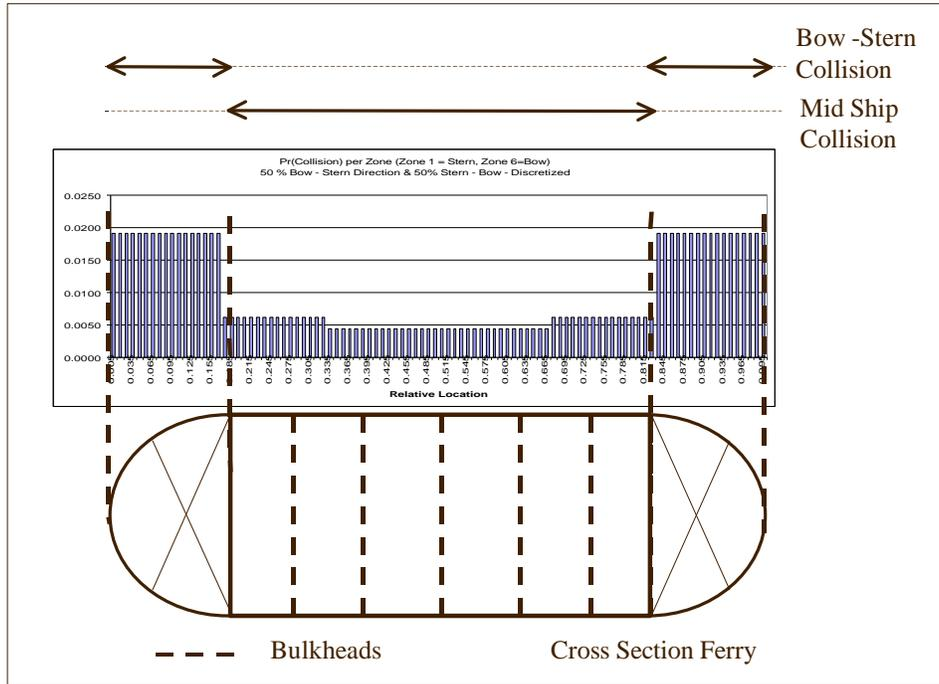
**Figure 19. Probability calculation of Mid-Ship Collision and Bow-Stern Collision**
