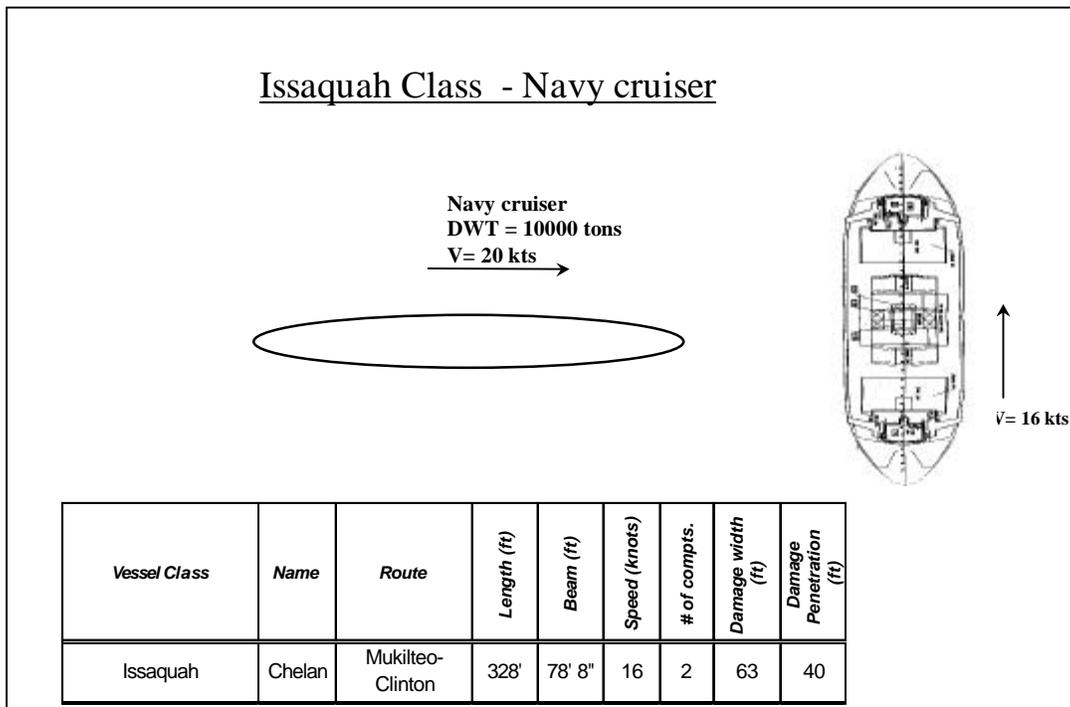
**Figure 13. A collision damage calculation based on a collision scenario with a navy cruises**
