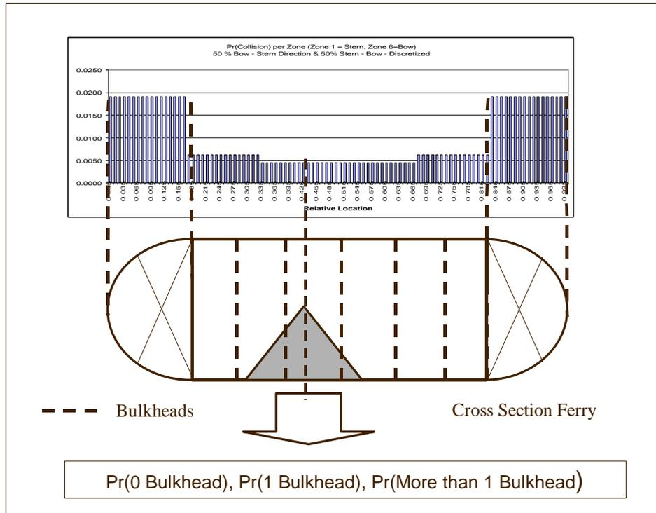
**Figure 24. Probability calculation of Bulkhead Damage Scenarios**
