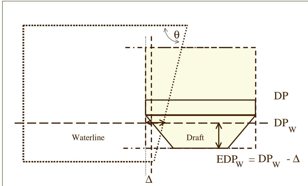
**Figure 14. Modified Analysis due to Vertical Bow Angle and Washington State Ferry Hull shape**
