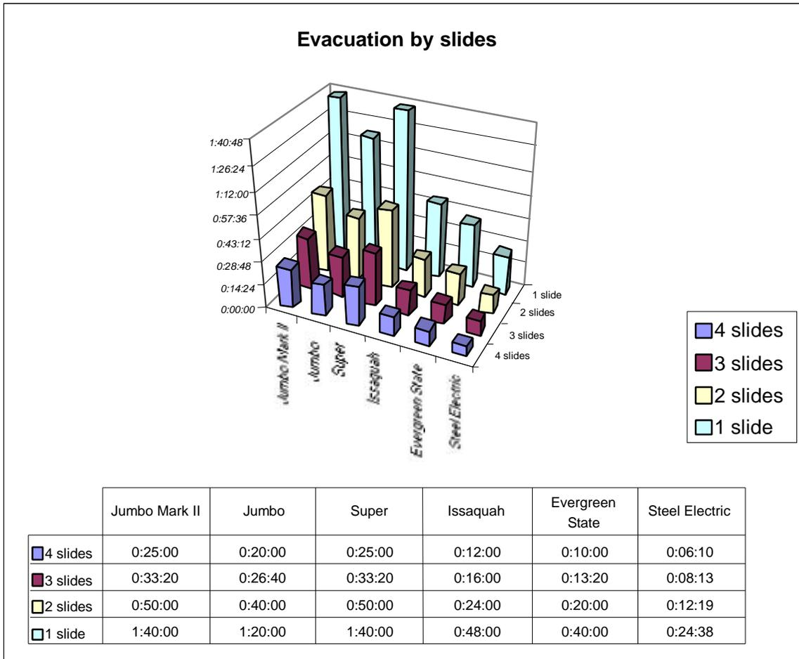
**Figure 17. Stage 3 Egress Completion Times (full capacity)**
