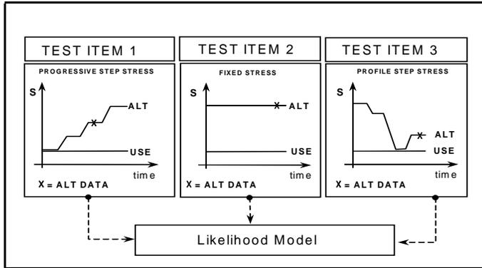
Figure 1. A Separate ALT Design for Each Test Item
