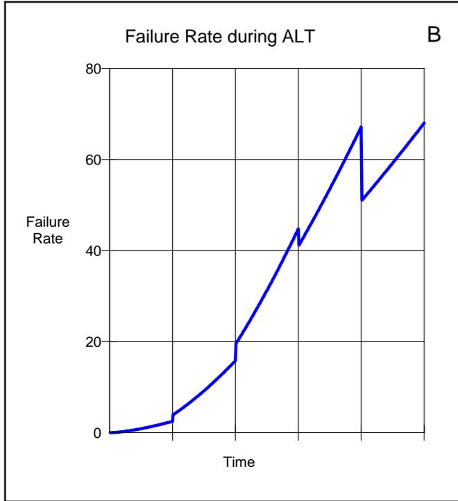
Figure 3. A: Selection of Failure Rate Sections from Weibull Failure Rate Functions B: Failure Rate During a Profile ALT by concatenating the failure rate sections selected in A.
