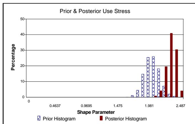
Figure 5. Prior & Posterior Shape Parameter - Interval Data.
