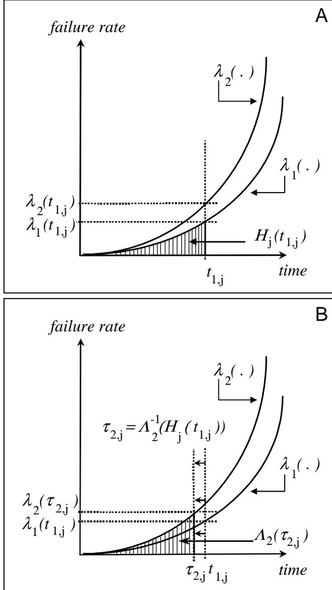
Figure 2. Failure Rate Construction Using Instantaneous Environment Changes. A: Failure Rate up to  $t_{1,j}$ ; B: Change Failure Rate to  $\lambda_2(\tau_{2,j})$  at  $t_{1,j}$  such that  $\Lambda_2(\tau_{2,j}) = H_j(t_{1,j})$ .
