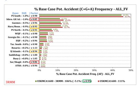
Figure 4-21. Relative comparison of POTENTIAL Accident Frequency by waterway zone. Red bars show the percentages by waterway zone for the USKMCA1600 What-If Scenario, greens bars show the percentages for the USKMCA1600-3RMM Scenario both in terms of base case percentages. Absolute differences by waterway zone and relative multipliers by waterway zone are provided in the y-axis labels.
