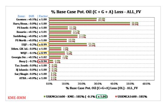
Figure 4-56. Relative comparison of POTENTIAL Oil Loss by waterway zone. Red bars show the percentages by waterway zone for the USKMCA1600 What-If Scenario, green bars show the percentages for the USKMCA1600-KME RMM Scenario both in terms of base case percentages. Absolute differences by waterway zone and relative multipliers by waterway zone are provided in the y-axis labels.
