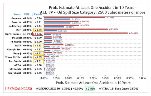
Figure 3-56. USKMCALN2250 relative comparison of probability estimate of at least one accident in a 10-year period by waterway zone for the POTENTIAL Oil Loss category 2500 m<sup>3</sup> or more.
