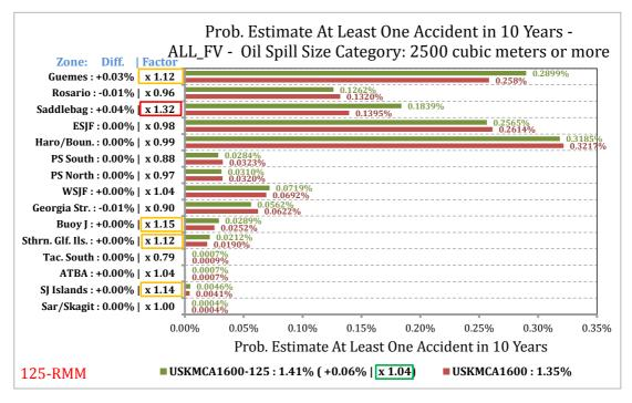
Figure 4-70. USKMCA1600-125 RMM Scenario relative comparison of probability estimate of at least one accident in a 10-year period by waterway zone for the POTENTIAL Oil Loss category 2500 m<sup>3</sup> or more.
