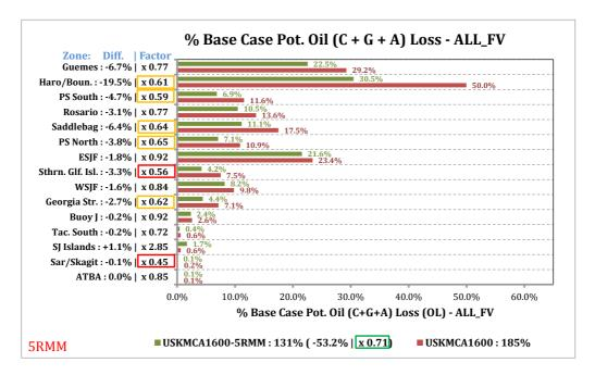
Figure 4-8. Relative comparison of POTENTIAL Oil Loss by waterway zone. Red bars show the percentages by waterway zone for the USKMCA1600 What-If Scenario, green bars show the percentages for the USKMCA1600- 5RMM Scenario both in terms of base case percentages. Absolute differences by waterway zone and relative multipliers by waterway zone are provided in the y-axis labels.
