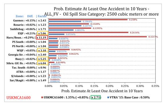
Figure 3-44. USKMCA1600 relative comparison of probability estimate of at least one accident in a 10-year period by waterway zone for the POTENTIAL Oil Loss category 2500 m<sup>3</sup> or more.
