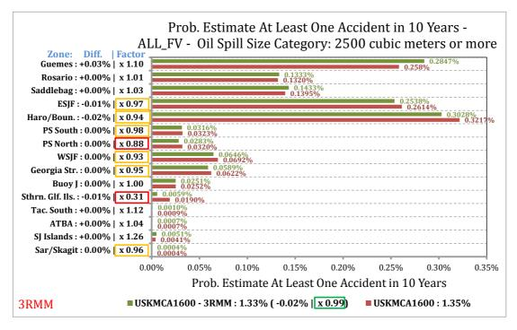
Figure 4-22. USKMCA1600-3RMM Scenario relative comparison of probability estimate of at least one accident in a 10-year period by waterway zone for the POTENTIAL Oil Loss category 2500 m<sup>3</sup> or more.
