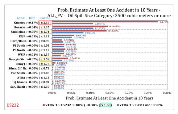
Figure 3-8. US232 relative comparison of probability estimate of at least one accident in a 10-year period by waterway zone for the POTENTIAL Oil Loss category 2500 m<sup>3</sup> or more.
