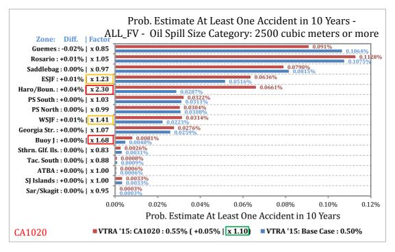
Figure 3-32. CA1020 relative comparison of probability estimate of at least one accident in a 10-year period by waterway zone for the POTENTIAL Oil Loss category 2500 m<sup>3</sup> or more.
