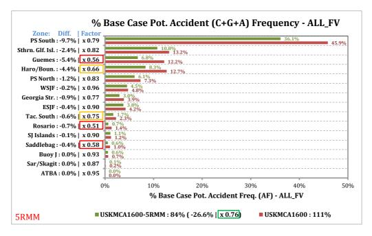
Figure 4-9. Relative comparison of POTENTIAL Accident Frequency by waterway zone. Red bars show the percentages by waterway zone for the USKMCA1600 What-If Scenario, greens bars show the percentages for the USKMCA1600-5RMM Scenario both in terms of base case percentages. Absolute differences by waterway zone and relative multipliers by waterway zone are provided in the y-axis labels.
