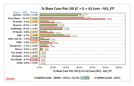
Figure 4-20. Relative comparison of POTENTIAL Oil Loss by waterway zone. Red bars show the percentages by waterway zone for the USKMCA1600 What-If Scenario, green bars show the percentages for the USKMCA1600-3RMM Scenario both in terms of base case percentages. Absolute differences by waterway zone and relative multipliers by waterway zone are provided in the y-axis labels.
