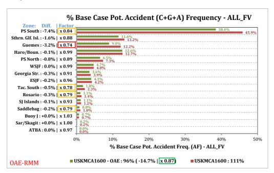
Figure 4-33. Relative comparison of POTENTIAL Accident Frequency by waterway zone. Red bars show the percentages by waterway zone for the USKMCA1600 What-If Scenario, greens bars show the percentages for the USKMCA1600-OAE RMM Scenario both in terms of base case percentages. Absolute differences by waterway zone and relative multipliers by waterway zone are provided in the y-axis labels.
