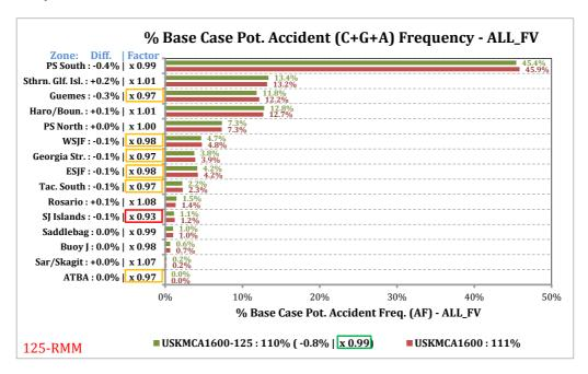
Figure 4-69. Relative comparison of POTENTIAL Accident Frequency by waterway zone. Red bars show the percentages by waterway zone for the USKMCA1600 What-If Scenario, greens bars show the percentages for the USKMCA1600-125 RMM Scenario both in terms of base case percentages. Absolute differences by waterway zone and relative multipliers by waterway zone are provided in the y-axis labels.
