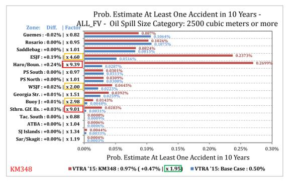
Figure 3-20. KM348 relative comparison of probability estimate of at least one accident in a 10-year period by waterway zone for the POTENTIAL Oil Loss category 2500 m³ or more.
