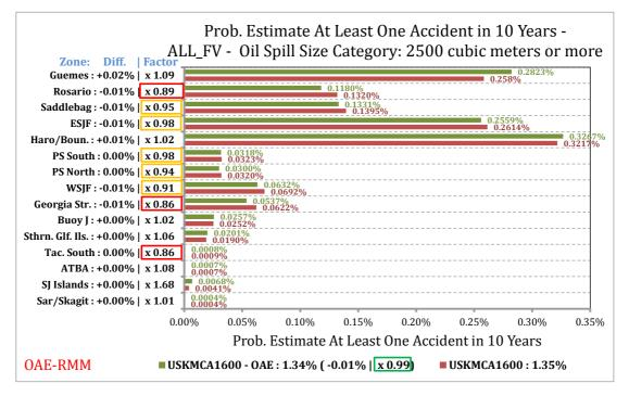
Figure 4-34. USKMCA1600-OAE RMM Scenario relative comparison of probability estimate of at least one accident in a 10-year period by waterway zone for the POTENTIAL Oil Loss category 2500 m<sup>3</sup> or more.
