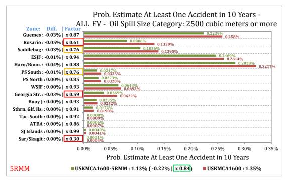
Figure 4-10. USKMCA1600-5RMM relative comparison of probability estimate of at least one accident in a 10-year period by waterway zone for the POTENTIAL Oil Loss category 2500 m<sup>3</sup> or more.
